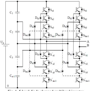
Fig. 1. 5 level diode clamped multilevel inverter
