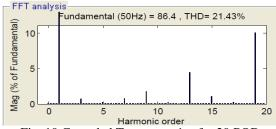
Fig. 10 Cascaded Type ma = 1;mf = 20;POD
