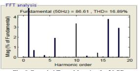
Fig. 8 Cascaded Type. Ma = 1;mf = 20;PD
