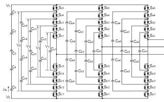
Fig. 2. flying capacitor multilevel inverter
