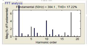
Fig. 6 Flying Capacitor ma= 1;mf = 20;PD
